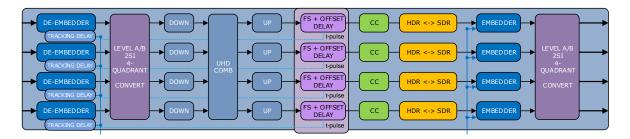
The NGH1616 has 16 processing paths, which include audio de-embedding, framesync, up/dn/cr conversion, UHD remapping, Proc Amp, embedding, audio gain/phase/delay and HDR<>SDR conversion functionality.
