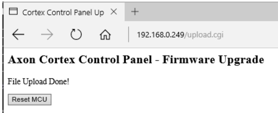
After doing this the browser will complete and the unit will reset itself after which the unit can be added back into the system by changing the IP address of the device in the system to the IP address of the unit.
