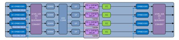
The NGP1600 has 16 processing paths, which include audio de-embedding, framesync, up/dn/cr conversion, UHD remapping, Proc Amp, embedding and audio gain/phase/delay functionality.
